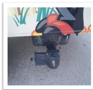
Liquid Waste Connection
